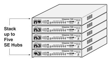
Fig. 3-4 Stackable SE Hub Configuration
